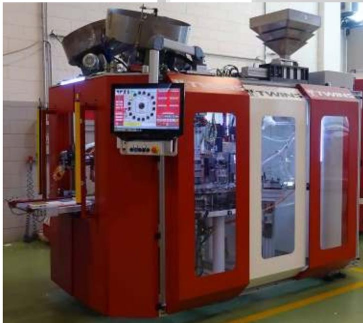
Strong and stable machine frame automatically loaded by centrifugal feeders, can unload the ammunition directly in the tray.
