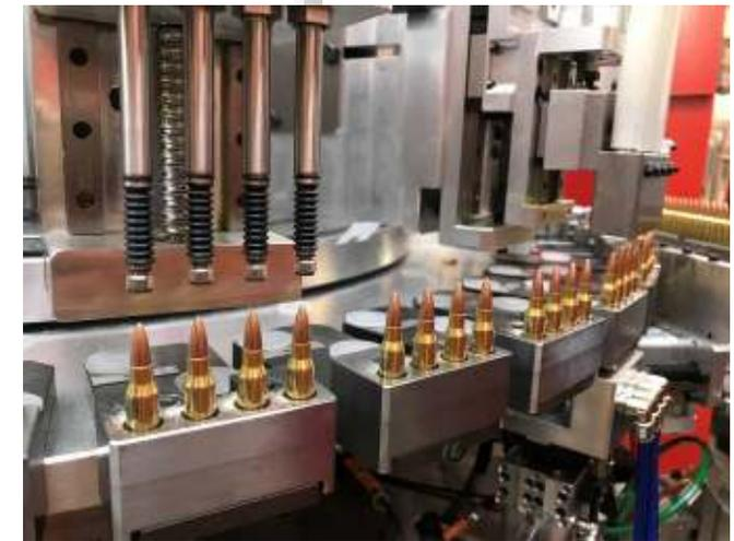
100% Electronic control of the bullet height (AOL) and the primer height, both are measured not just as ok or not ok, their measure is stored in the machine database, pieces by pieces, allowing the statistical analysis.
