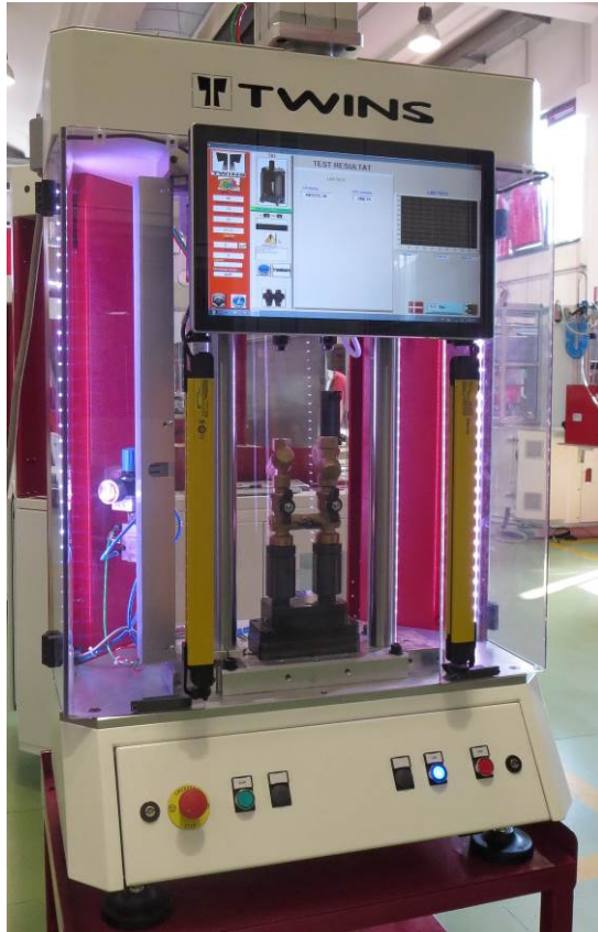
Pneumatic system and photo shields
