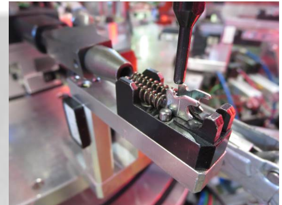
Spring test & loading with pre-compression 100%
