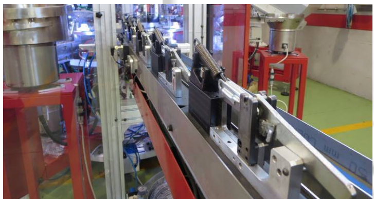
Flexible pallet line to join the cam group, satellite machine with the main assembly machine.
