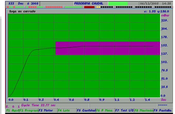
Real time Leak test graphic
